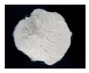
Yttrium stabilized zirconia powder is a highly advanced ceramic material that has numerous applications in various industries. It is a composite material that is made by adding yttrium oxide to zirconia powder. The addition of yttrium oxide stabilizes the zirconia crystal structure, making it more resistant to cracking and other forms of deformation.
